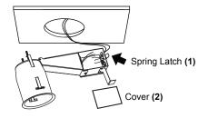
5. Connect the wires based on diagrams below. Close the junction box.
