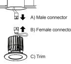
For the adjustable trim (LD2A, LD2B, LD2D, LD2E, LD3A, LD3B), choose aiming angle then tighten screws to lock into position.
