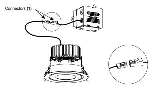
Push the spring loaded clips in vertical position and insert the fixture in the ceiling. Release the clips and the fixture will be pulled flush to the ceiling.
