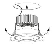
The incremental adjustment (2.5 degrees each) of the adjustable trim is accomplished by simply pressing the center part flange towards the desired angle.
